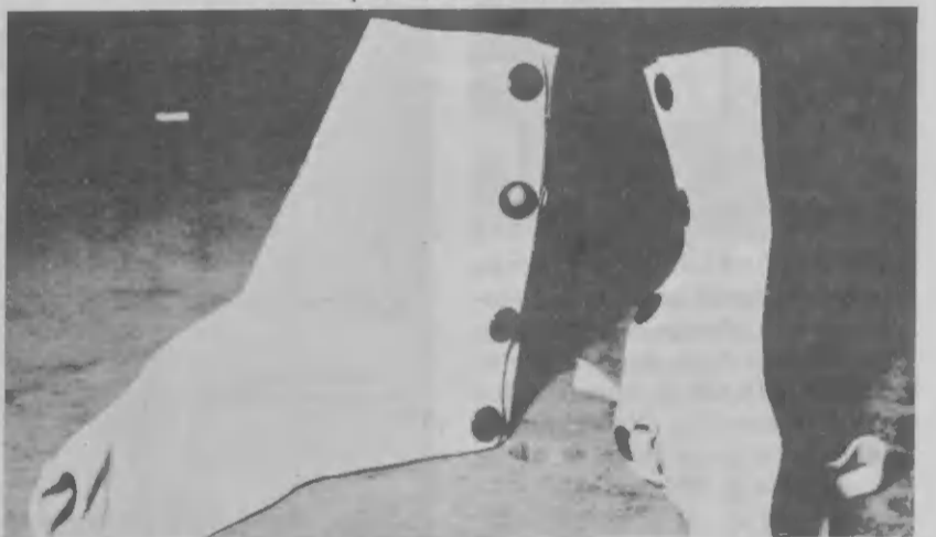
THESE ARE not leggings of the marines, but leg protection used by welders. ESAKINAN na ta polaina di mariniers, pero proteccion pa pia usa door di weldernan.
